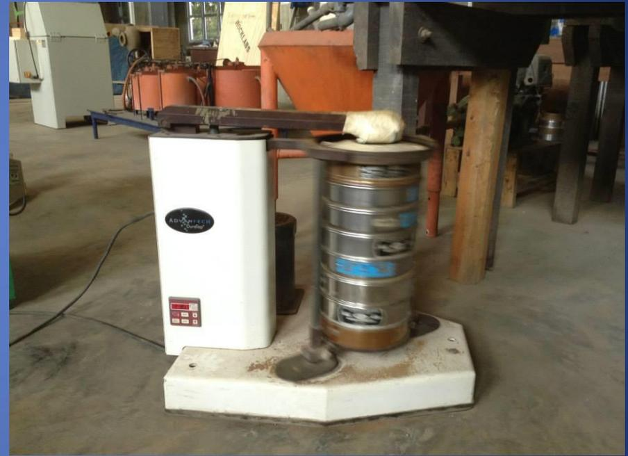
*Figure 4. Particle size reduction by Ball Milling, and RoTap and sieving.*
