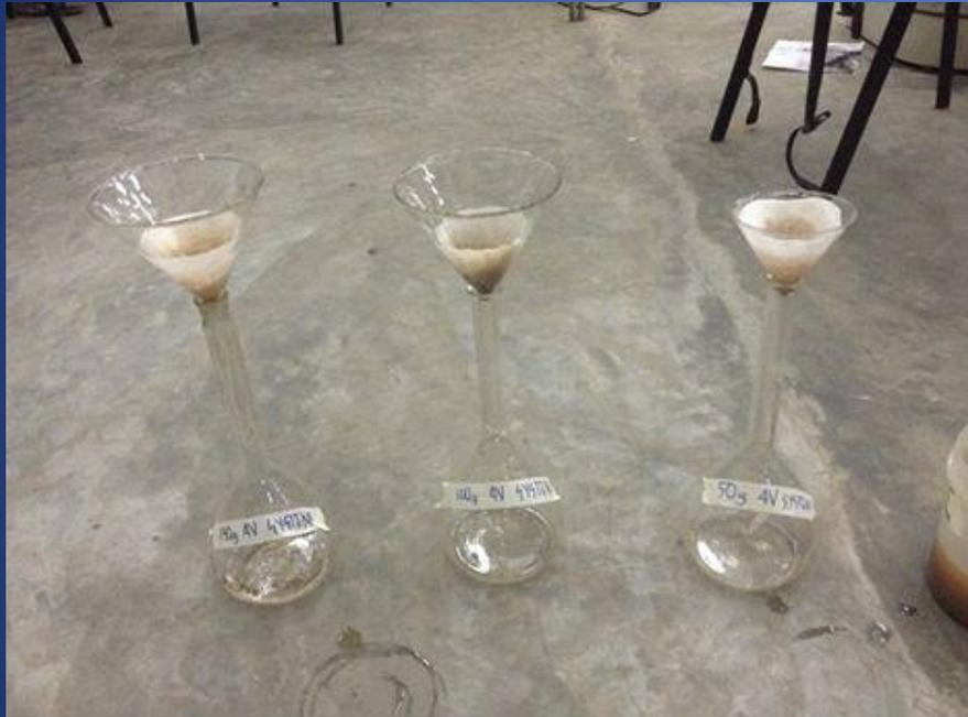
*Figure 7. Silt collected from the system is decanted and filtered*
